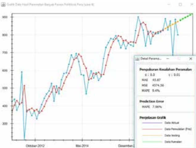
Fig. 4. Graph and forecast error rate from the way of initial smoothing value determination 4
