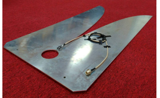
Fig. 10. Antenna realization according to the design parameter, which is ready for real-field measurement and applications.
